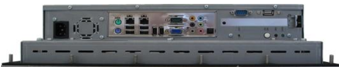
Bottom IPPL Panel - PC with one PCI Slot
