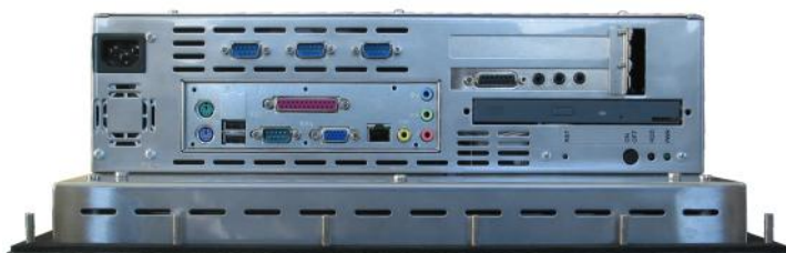
Bottom IPP-15.. Panel - PC with CDRW Drive and 2 PCI Slots
